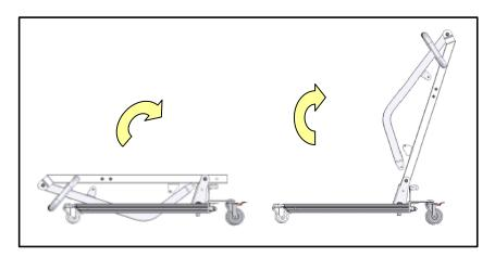
**Step 1.** Engage the brakes. Remove the bolts from the bottom of the mast and base. Pull the Mast, Boom and Spreader Bar to an upright position. Re-insert the bolts into the holes at bottom of the mast and tighten the nuts.
