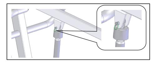
**Step 5.** Attach the spreader bar to the boom and insert pin. Insert keeper ring to secure spreader bar to boom.
