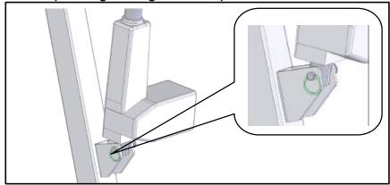
**b.** Attach the top of the Actuator to the bracket on the Boom and insert pin. Insert keeper ring through hole in pin to secure actuator to upper bracket.
